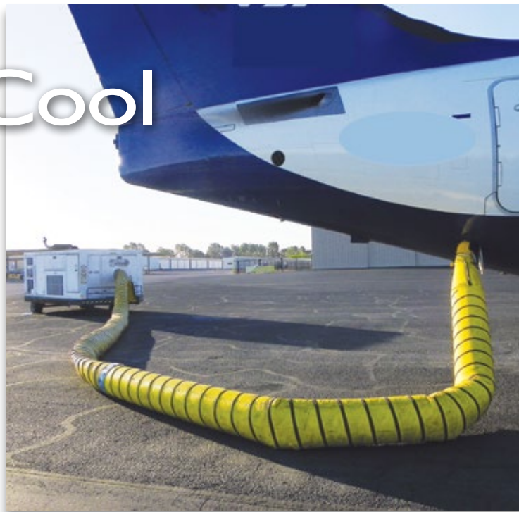
A heavy duty ground cooling unit preparing a passenger aircraft for flight from Tucson, Arizona.
