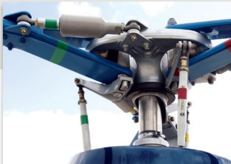
Above: The rotorhead is aluminium alloy with magnesium forging surrounded by a fibreglass 'safety belt' for protection if the head cracked.
