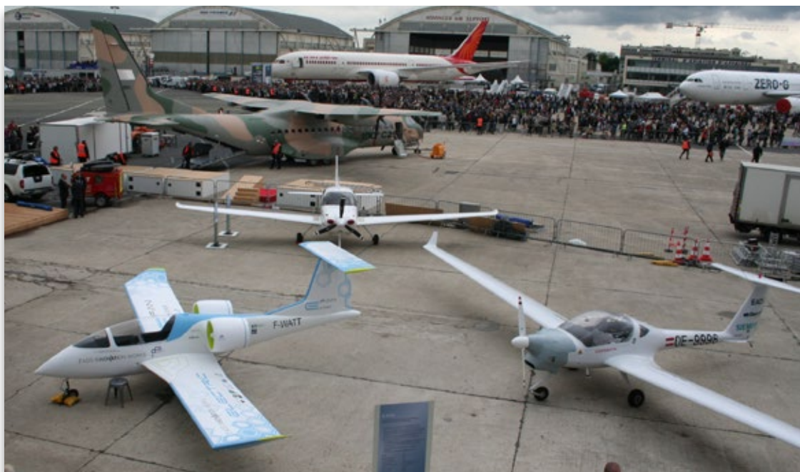
Left: The E-FAN on the left side and on the right the DA36 E-STAR two experimental electric planes developed by Diamond Aircraft, EADS and Siemens.
