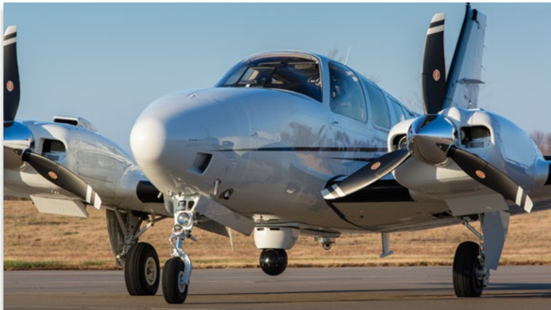
The 230-HD EO/IR camera on the undercarriage of the Baron G58.
