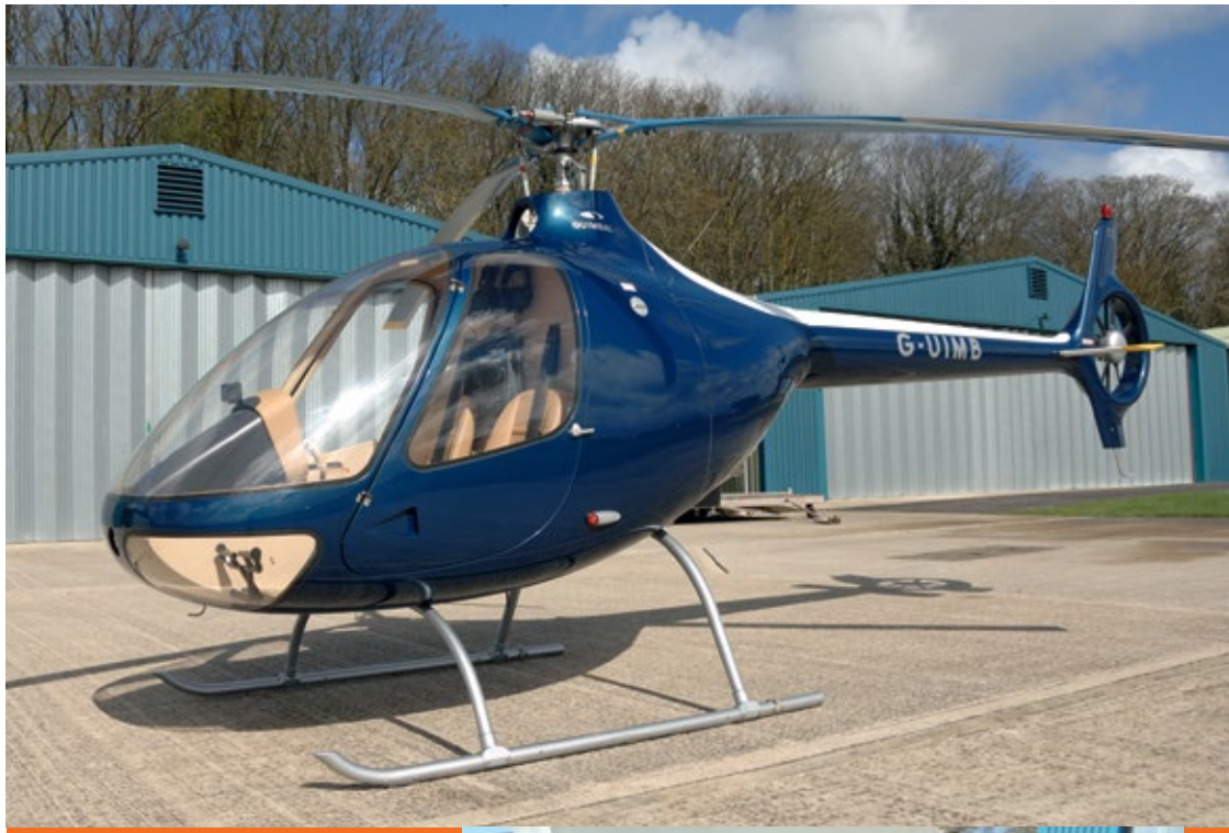
Above: The landing gear is composite and because there are no oleos there is a damper between the skids and the body of the G2.
