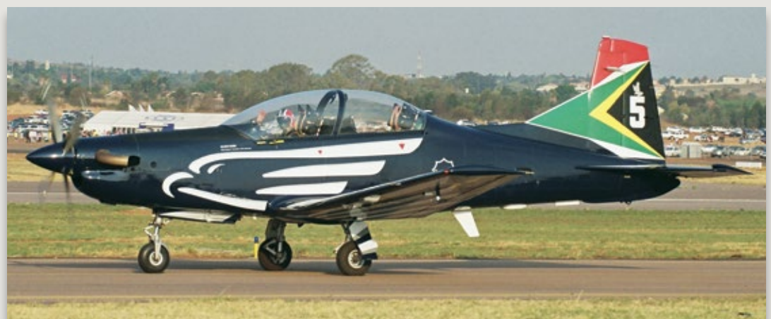
The easiest means of identifying a modified PC-7 Mk II is evident in this view of serial 1015 seen at Africa Aerospace and Defence 2012 at Air Force Base Waterkloof on September 22. The GPS antenna is clearly visible on the front top of the vertical fin, the more prominent wing root fairings less so - Pic Clinton Barnard.
