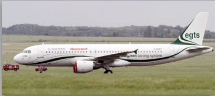
The Safran EGTS, the Electric Green Taxiing System allows a significant gain in fuel savings.
