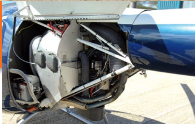
Right: The engine is a standard Lycoming 360, fitted with one magneto and one plasma ignition system.
