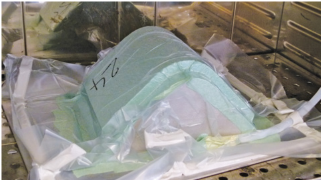
Figure 14: Vacuum bag thermoforming an S-shaped part from TegraCore™ PPSU foam (600 × 900 mm/2.0 × 3.0 ft)
