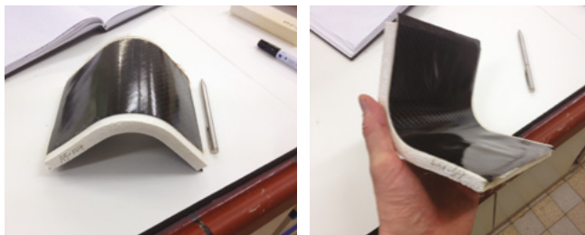
Figure 17: TegraCore™ PPSU foam board with a 1-mm (0.04-inch) thickness shaped into a rectangular pipe using Udel® PSU film as a tie layer
